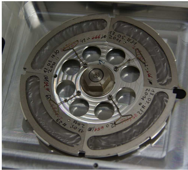
Figure 9: One of the TASCA target wheels. The diameter of the wheel is 100 mm.
