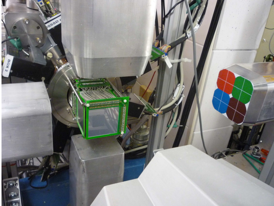
Figure 1.2: The TASISpec setup: The ions enter the “box” of silicon detectors seen in the left part of the figure. The DSSSD is the detector that is facing the camera, and the other two detectors that are seen to form the sides of a box upstream of the DSSSD are SSSSDs. During normal operation, there is a cap that covers the silicon detectors. The three detectors on the left, top and bottom of the silicon detectors are germanium detectors of CLOVER type. The coloured detector to the right shows how the four Ge crystals are arranged inside a CLOVER detector. The lower part of the photo shows the CLUSTER germanium detector, which contains 7 crystals. This detector is placed behind the DSSSD.
